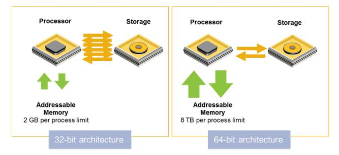
As this figure shows, advantages of 64-bit architecture include:
