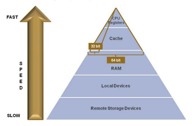
Local devices are onboard storage units, such as hard drives, and remote storage devices are removable storage, such as CDs, DVDs, and tape.
