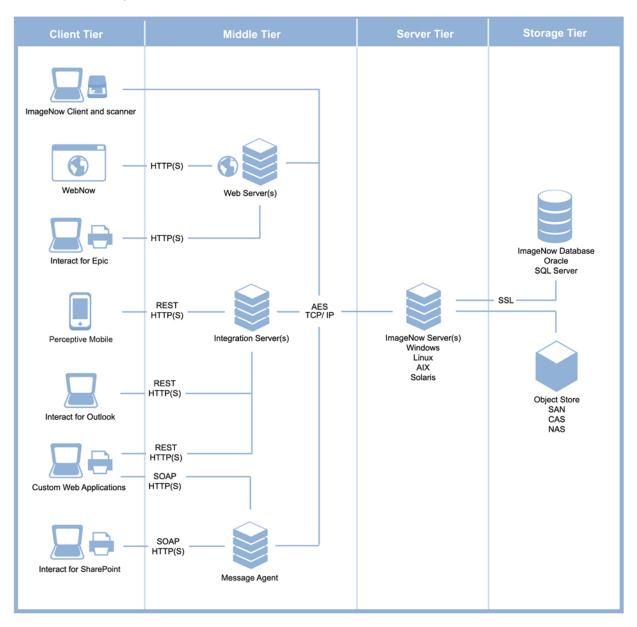
Communication between Perceptive Content Server and other components, such as Perceptive Content Client and WebNow occurs over TCP/IP using a socket-based communication protocol defined by Perceptive Software to achieve best possible performance. The socket communication consists of a series of calls that the clients use to request information from the Perceptive Content Server.
