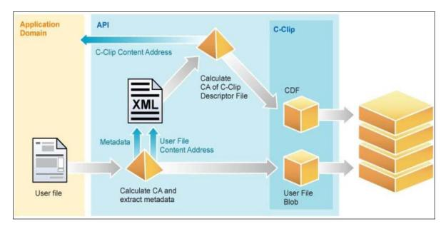
A benefit of storing BLOBs of content is that it allows Centera to detect when duplicate content reaches the system. Only one instance is ever stored in addition to a mirror copy. Perceptive Content communicates with EMC Centera by referencing the C-Clip content address only. For customers running Perceptive Content prior to obtaining EMC Centera, Perceptive Content can copy pre-existing document objects.
