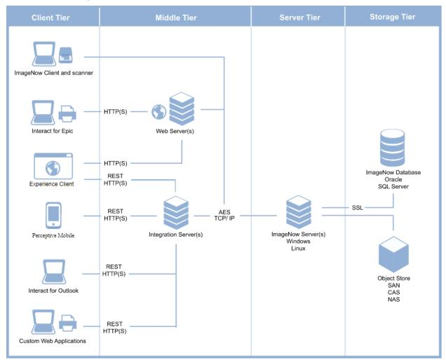
Communication between Perceptive Content Server and other components occurs over TCP/IP using a socket-based communication protocol defined by Perceptive Software to achieve best possible performance. The socket communication consists of a series of calls that the clients use to request information from the Perceptive Content Server.
