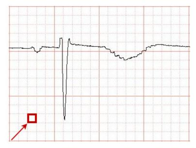
A group of 5 horizontal boxes, bordered by a thick line, represents a 5 mm interval or 0.2 seconds (200 ms).
