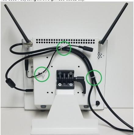
**3.** Tie the cables using the tie wraps (p/n 400-00012-00). Use the following image as a guideline for how to manage the cables.
